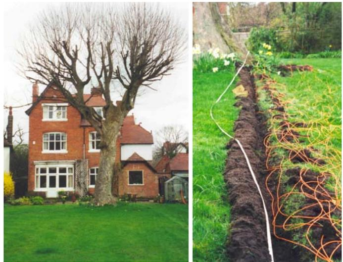
Dr. Ron Barker applied water to an area of the ground in the vicinity of a mature and pollarded Sycamore in his rear garden and measured infiltration rates over time using ERT.
